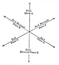
F1G. 105. Diagram of three-phase, six-phase transformation, by reversal secondary terminals of transformers.
